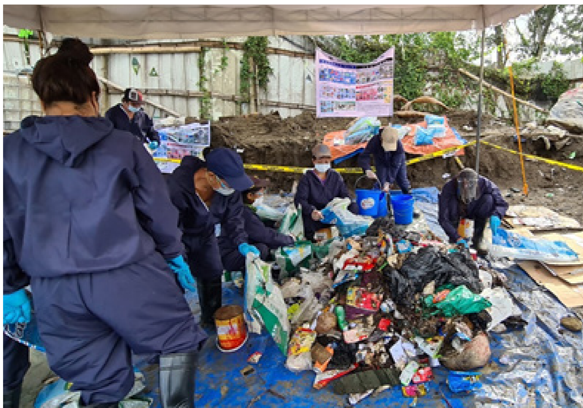
Figure 29. Sorting of Quartered Waste Sample last September 27, 2021
