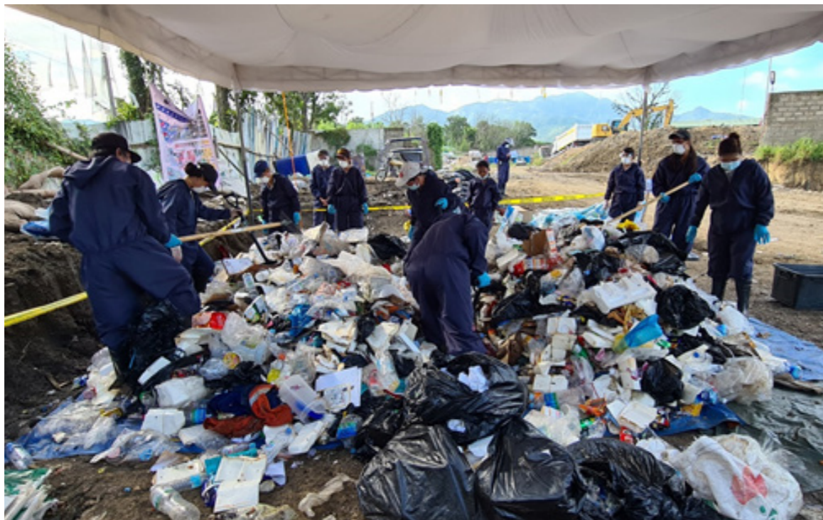
Figure 28. Sorting Area and Quartering of Waste Sample at the Landfill last September 28, 2021
