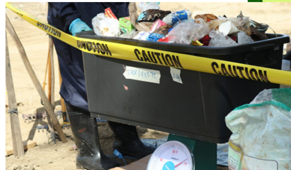
Figure 30. Bulk Density Measurement last September 26, 2021
